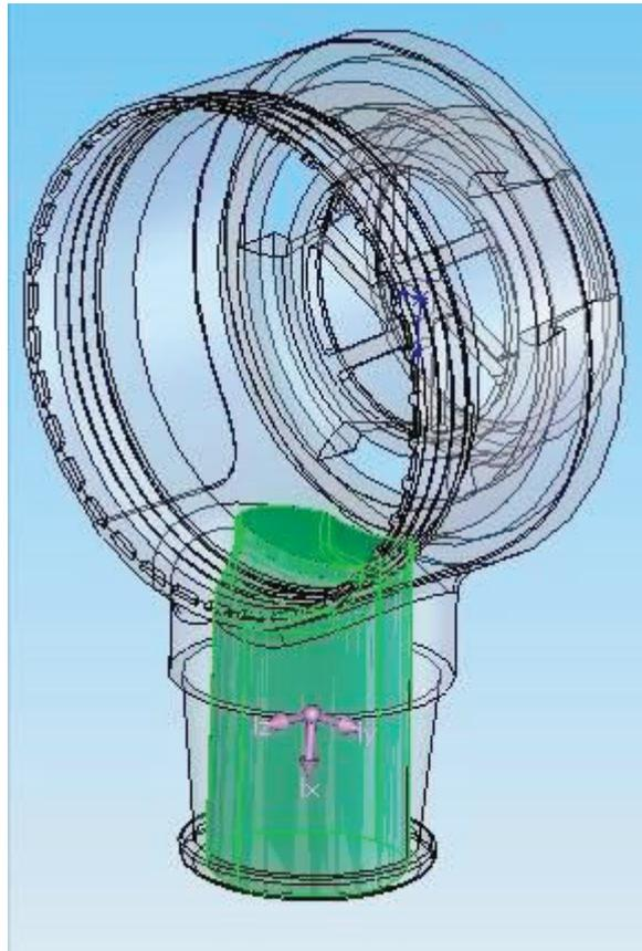
Figure 9: 3D illustration of the T-Valve.
